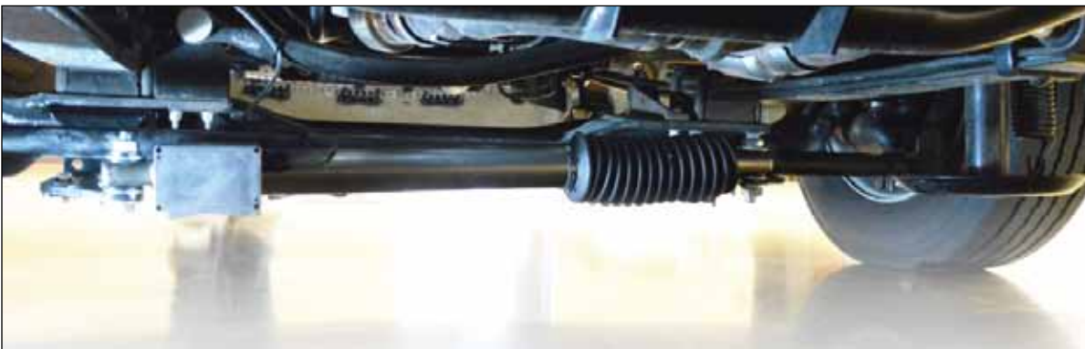
The Blue Ox TruCenter steering stabilizer consists of an electronic module that controls the behavior of a spring. The passive system helps in providing directional control.
